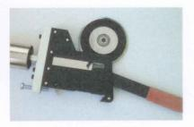
Insert into knife holder as shown in picture and apply downward pressure. This will release the blade without causing damage.
